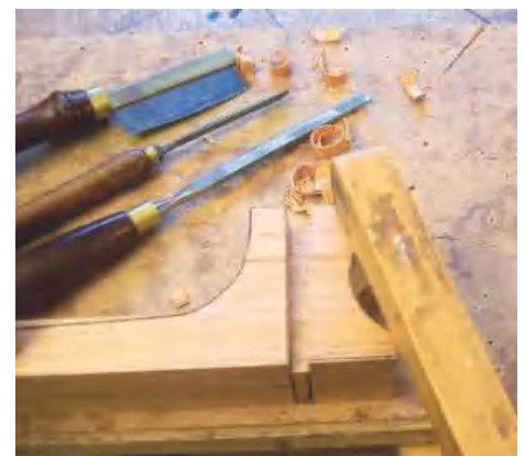
▲ Pic.19 The wedge slots chiselled out
